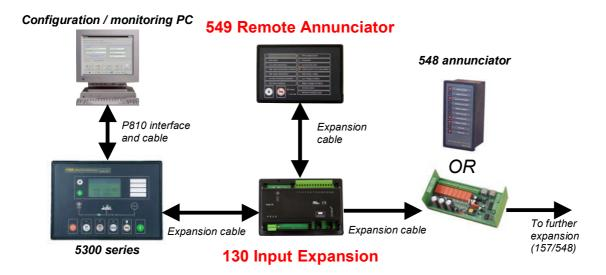
$oldsymbol{\Omega}$ NOTE:- Previously, the 53xx expansion port was used solely for output expansion. For this reason, modules manufactured prior to the release of the P130 input expansion module may be marked as: 157/548 ✓ These 'early' modules are NOT compatible with the P130 input expansion module.
