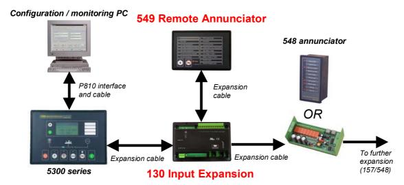
$oldsymbol{\Omega}$ NOTE:- Previously, the 53xx expansion port was used solely for output expansion. For this reason, modules manufactured prior to the release of the P130 input expansion module may be marked as: 157/548 ✓
